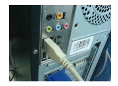
★ Please use the same USB2.0 port every time. Using on a different USB2.0 port requires reinstalling or updating the driver again to make the camera work rightly. If not, it will influence the performance of the camera, and cause the live image displays drag, for there is another system driver, and the system set it as default driver.
